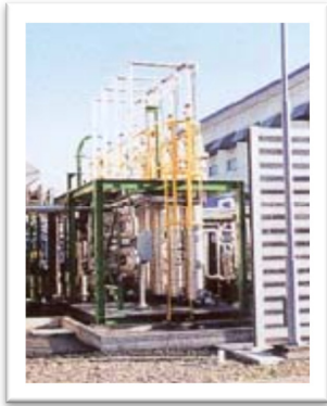
Membrane System for natural gas treatment installed in Japan
